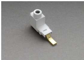
33907 000 connecting terminal, front connection for 3-pole comb-type busbar 35 mm 2 , suitable for NH-fuse-switch- disconnector size 000 with box terminal 4 - 35 mm 2
